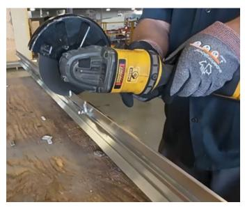
12. After marking the intended locations to notch for either your outside corner or termination extrusion, clamp the marked extrusion onto a workbench and cut the notch out of the extrusion using a grinder or other cutting tool. Ensure appropriate PPE is being worn when completing this process.
